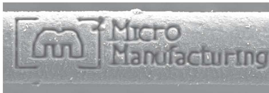
Human hair with laser micromachining.
