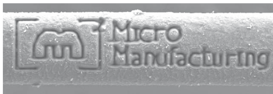
Human hair with laser micromachining.
