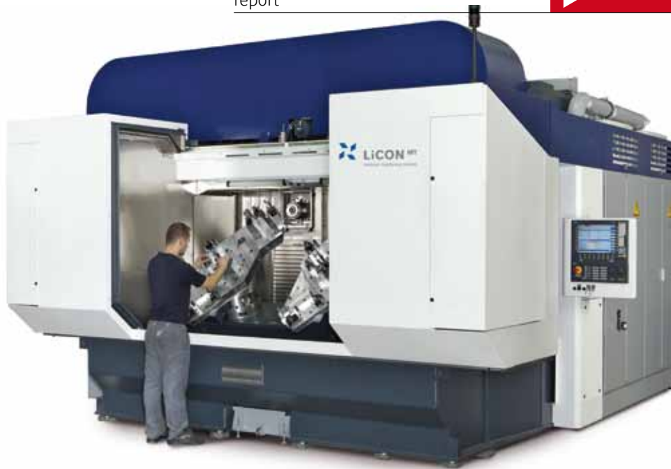
LiFLEX II 1066 is the largest among horizontal double spindle machines in the Licon portfolio. Workpieces with a size of up to 1,000 mm can be processed in one setting in this machine.
