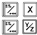
On the 20iE model, it could occur that the installation parameter PAR11(1) has been set to "0" for this key to independently affect each axis so that one axis can display its position in incremental mode while the other does this in absolute. In this case, to change the display mode for a particular axis, press one of these sequences.
