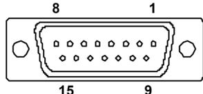
X4 is a 15-pin female SUB-D connector to connect 4 opto-coupled digital inputs and 6 opto-coupled digital outputs with solid state relays with normally open contacts that may be used to activate relays, beacons, etc.
