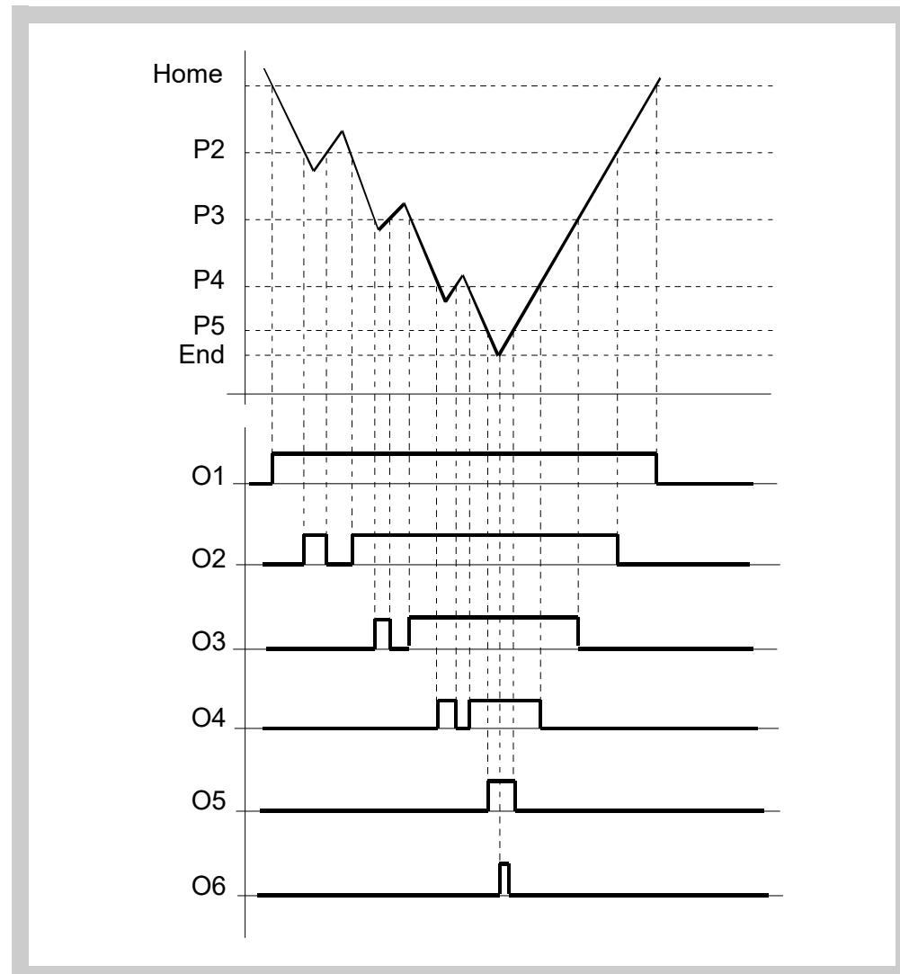
PAR20 bit 4 = 1 (the outputs are deactivated when reaching the home position).
