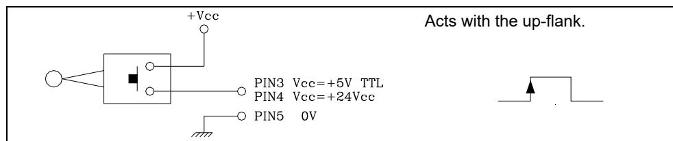
Probe with "normally closed contact" output.
