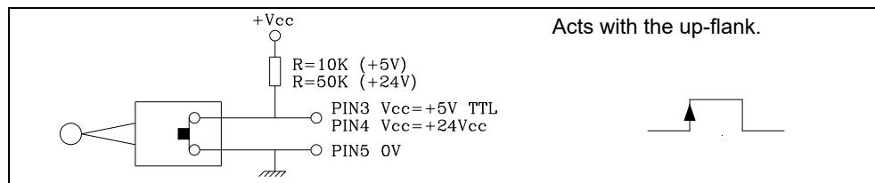
Interface with an open-collector output. Connection to +5 V.
