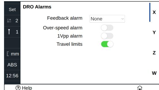
**3- Feed rate overrun alarm:** When set to YES, an alarm is issued over 200 kHz.
