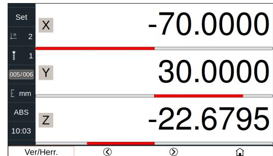
Once positioned at the drilling point, touch the surface with the tool. Press the Z axis key. The Z axis display reads zero.
