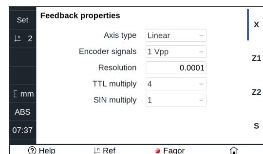
**2- Type of encoder signal:** TTL, 1 Vpp orSSI.
