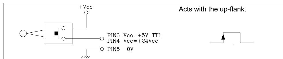
Probe with "normally closed contact" output.
