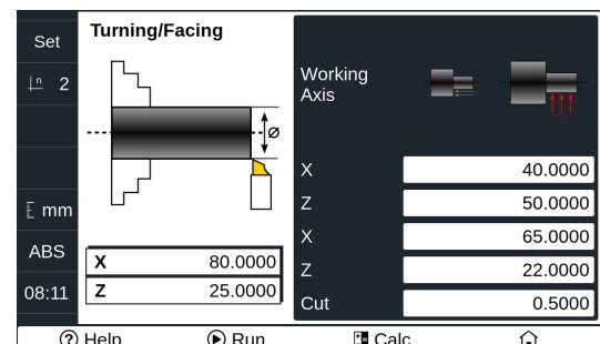
**Cut:** Enter cutting pass in mm. The DRO will use this value also as the safety distance to withdraw after each pass.
