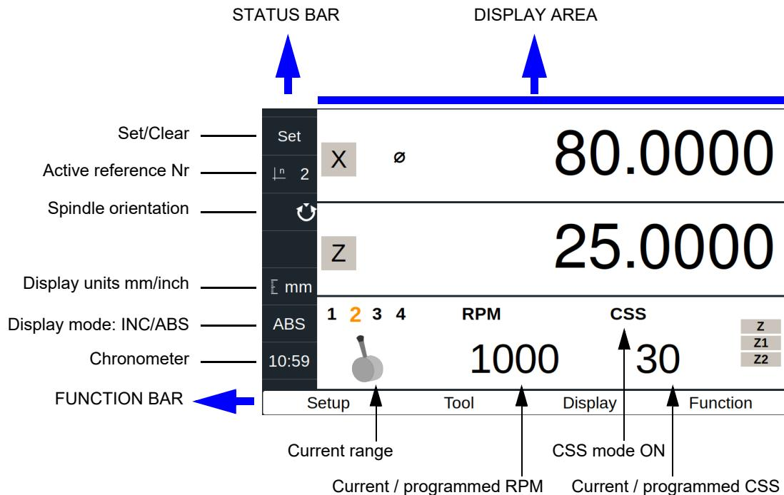
When the spindle is off, the RPM and CSS displays show the programmed values.
