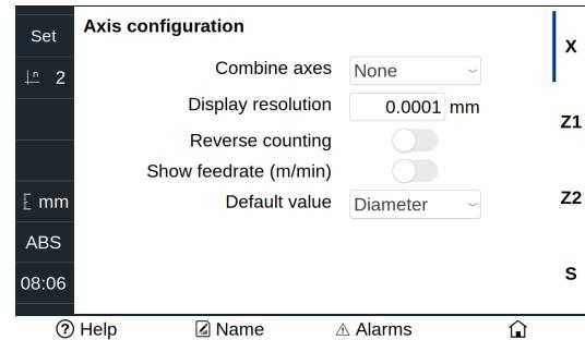
**3- Reverse the feedback reading (pulse counting) direction:** Yes or NO. Factory setting: NO.
