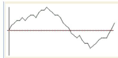
**Note:** The maximum slope for the compensation graph is  $\pm 0.8$  mm/m.
