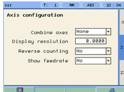
**3- Reverse the feedback reading (pulse counting) direction:** Yes or NO. Factory setting: NO.
