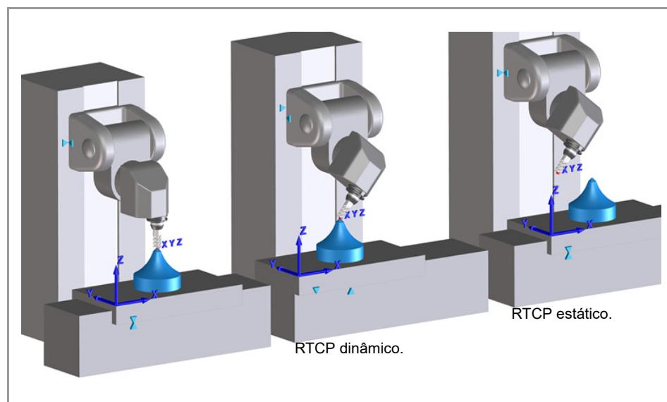
**USINAGEM EM 5 EIXOS COM RTCP (ROTATING TOOL CENTER POINT)**
